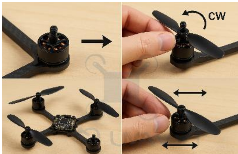
Figure 4.9. Drone Propeller Assembly - Direction and Tightness Control
