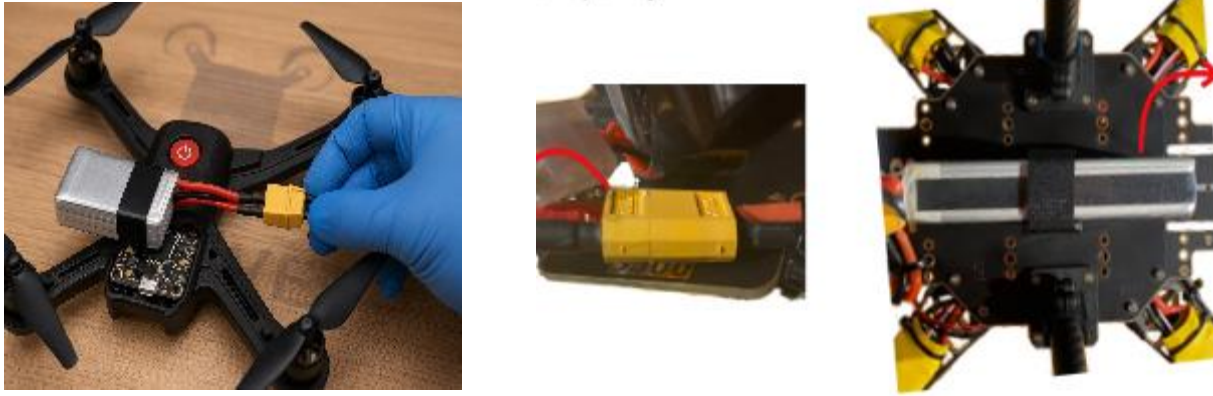
Figure 4.5. De-energising the Drone for Safe Intervention
