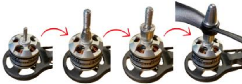
Figure 4.7 Drone's Electric Motor - Main Actuator Providing Propeller Movement
